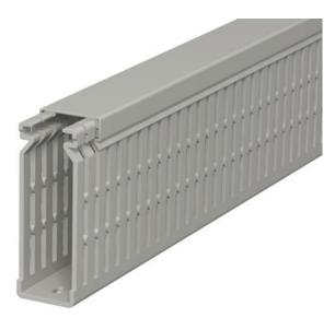
Wiring duct, incl. cover and base perforation, for horizontal and vertical routing of electrical cables in the switchgear cabinet. Designed as a metric duct. The nominal dimension of the system size corresponds to the internal dimension of the duct. Retainers are broken out without tools. The flush-floor routing of cables is possible through predetermined break points. Tapering in the side slots prevents the cables from falling out. Tested to DIN EN 50085-2-3. Special lengths on request.
