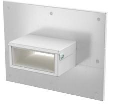
Wall connection collar, 4-sided, with integrated seal for PYROLINE® Rapid PLM installation duct. For mounting in the area of wall and ceiling connections as well as wall penetrations. Can also be used as 3-sided wall connection collar for direct wall or ceiling mounting of the duct.
