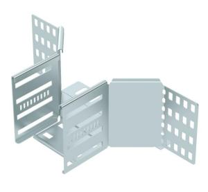
Add-on tee for the creation of a horizontal branch or cross-over, fitting for lock and screw-on cable trays of side height 110 mm. Screwless mounting with double clamps or screw connection with FRS truss-head screws and M6 combination nuts. Can be used in indoor areas. Fastening material must be ordered separately.
