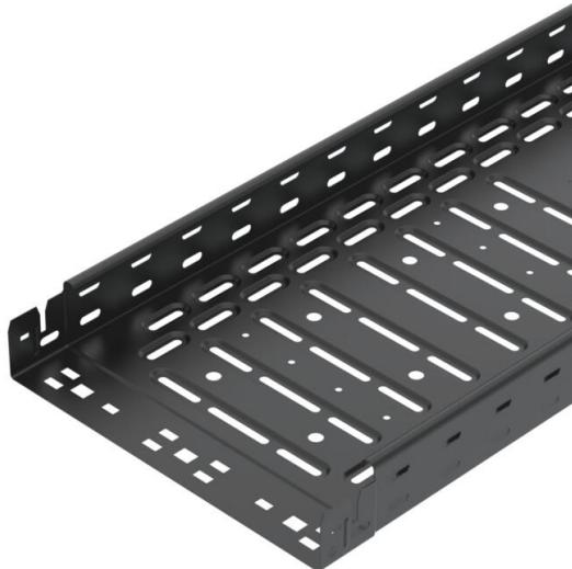
Cable tray with integrated quick-fastening system. Strip-galvanised surface, visible areas powder-coated in jet black (RAL 9005). Continuous side perforations of 7 x 20 mm for the installation of additional connection and mounting components. With 11 mm perforation in the base for direct threaded rod suspension. Usable length 3,000 mm.
