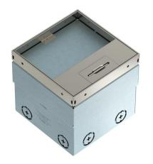
Square floor socket for use in dry-care cavity and screed floors in indoor areas. Installation housing with pre-marked insertion openings for pipes (M20/M25). Cover adjustable to top edge of floor covering using four height-adjustment supports. The minimum installation depth is 110 mm, the height-adjustment range is +25 mm
