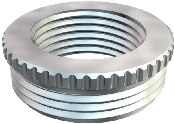
Reduction (Part H) to DIN 46320, with Pg thread to DIN 40430, as a transition from a PG thread hole to a smaller cable gland.
