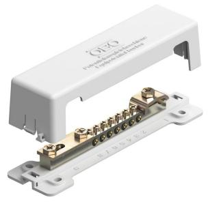
The OBO Green equipotential busbar is a solution manufactured from cellulose acetate CA for the installation of the equipotential bonding according to DIN VDE 0100-410/-540 and lightning protection equipotential bonding according to DIN VDE 0185-305. The basic material is widely used in the paper industry.
