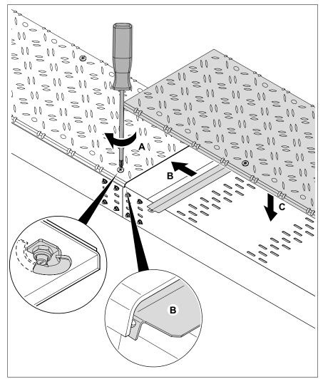
Figure 19: Mounting of cover with turn buckle
