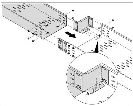
Figure 8: Changing the cable tray width
