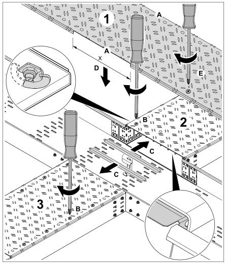
Figure 21: Mounting the cover on a cross-connection
