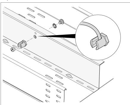
Figure 13: Mounting of the earthing terminal on the Z barrier strip
