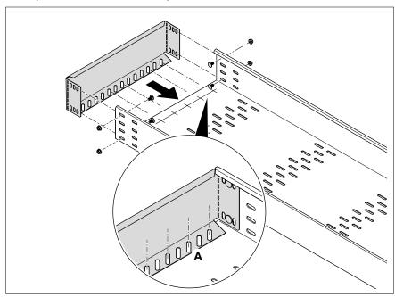
Figure 9: Closure of open ends
