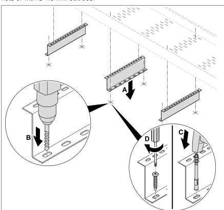
Figure 2: Mounting of support profiles
