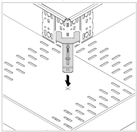
Figure 14: Installation of cover support
