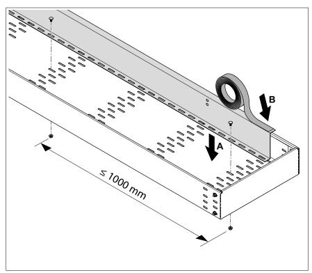
Figure 10: Barrier strip mounting
