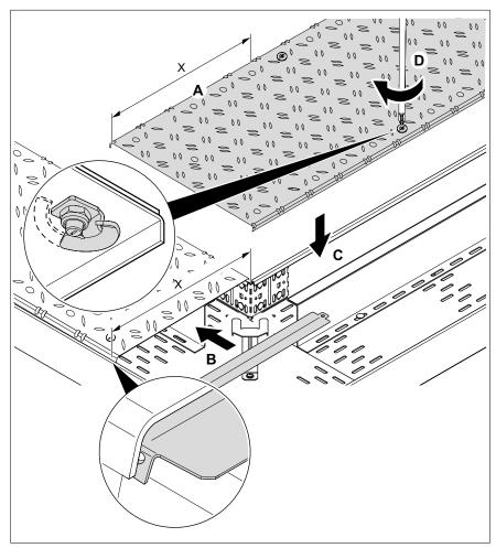
Figure 20: Mounting the cover on a corner connection
