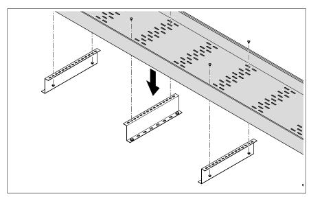
Figure 4: Mounting on support profiles
