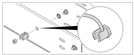
Figure 12: Mounting of the earthing terminal on the cable tray rail
