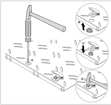
Figure 18: Mounting the turn buckle, type DRL H FT
