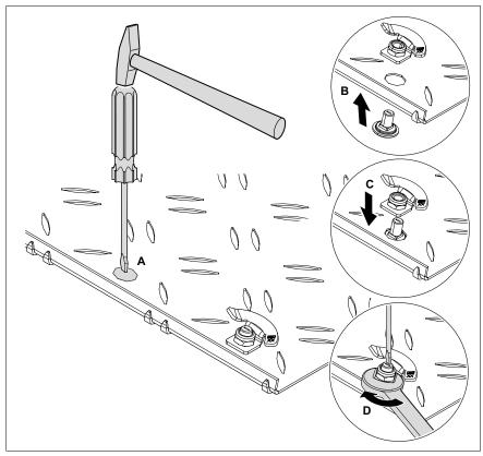
Figure 17: Mounting the turn buckle, type DRL H A2
