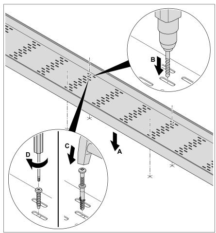
Figure 3: Mounting directly on the ground
