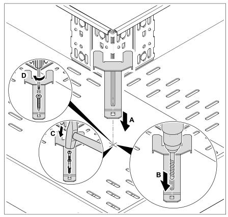
Figure 15: Direct floor mounting of the cover support
